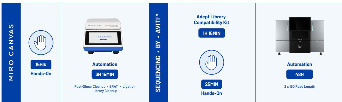
**Figure 1.** Experimental Workflow. The Miro Canvas automates all the PCR-Free Whole Genome Sequencing Library Prep steps following reaction setup, including: Post shear bead cleanup, end repair and A-tailing, adapter ligation and two back to back bead cleanups. Downstream library circularization using the Adept Library Compatibility Kit was manually performed.
